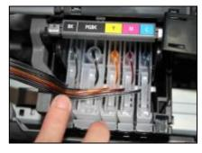
Please make sure that every cartridge is well installed according to the color label.
